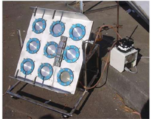
Fig 3. Nine Cell Reactor for purification of water.
